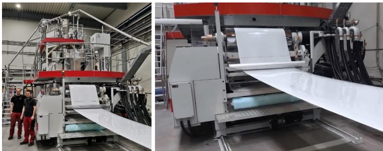
rPET 100 sheet production on a viscoSHEET extrusion line
